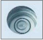
the up-front level indicator helps to ensure that the balance is level prior to each use.
