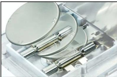
AutoCal™ internal calibration system automatically calibrates the balance when it senses a temperature change significant enough to affect the weighing accuracy.
